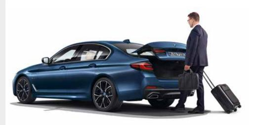
The **Comfort Access** with smart-opener makes it possible to open all four vehicle doors, including the luggage compartment, without using the key. This equipment includes contactless opening of the bootlid with a quick wave of the foot under the rear bumper.
