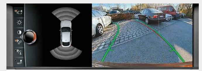
**Parking Assistant with Rear View Camera** makes parking and manoeuvring the vehicle easier. The Parking Assistant with linear guidance parks the vehicle automatically, parallel or perpendicular to the street. If the driver parks manually without the help of the Parking Assistant, Active Park Distance Control (PDC) offers additional protection against damage with the Lateral parking aid.
