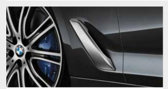
The **Air Breather** channels air to the front wheels, reducing air resistance, fuel consumption and  ${\rm CO_2}$  emissions.
