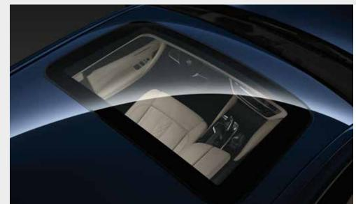
The **Electric Glass Sunroof** with slide and lift function, including an electric sliding interior roof, anti-trap protection, as well as comfort opening and closing, allows the airflow to be individually regulated to create a pleasant interior climate.
