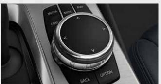
The **iDrive Touch Controller** with direct menu control buttons, eight functional bookmarks and voice control makes operation intuitive by allowing you to enter the address of your destination in handwriting on its touch-sensitive surface.
