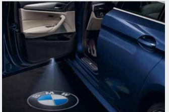
The Innovative BMW Door Projectors. The innovative door projectors are automatically activated when the doors are opened. They project an image onto the ground next to the car using an interchangeable slide
