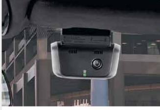
BMW Advanced Car Eye 2.0. A highly sensitive full-HD camera that captures events in front and behind the car, even when it is parked. In the event of disturbances and extraordinary movement outside the vehicle, the camera automatically records the situation in order to document possible accidents or (attempted) break-ins.
