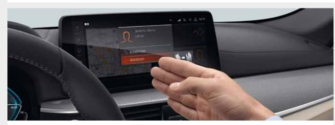
With **BMW Gesture Control**, selected functions can be operated by means of defined hand movements. Simple gestures such as 'swiping' or 'pointing' are identified in the recognition area above the centre console and trigger functions such as accepting or rejecting an incoming telephone call, proceeding or cancelling navigation as well as starting and ending voice recordings.
