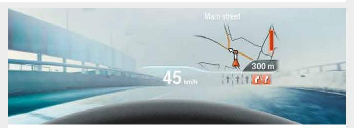
**BMW Head-Up Display** offers a full-colour projection of driving relevant and situational information onto the windscreen with improved resolution of  $800 \times 400$  pixels.
