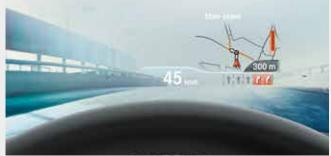
The **BMW Head-Up Display** offers a full-colour projection of driving relevant and situational information onto the windscreen with improved resolution of  $800 \times 400$  pixels.
