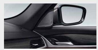
The **Harman Kardon Surround Sound System** with a powerful 464-Watt digital amplifier, vehicle specific equalising, 16 loudspeakers, including 2 with Chrome surround, a center speaker and surround mode create an aural experience of the highest intensity.
