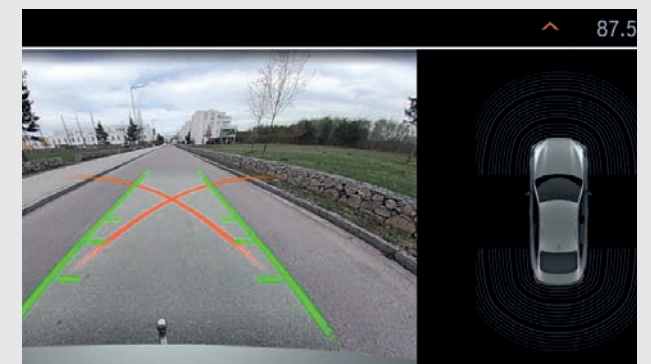
The Reversing Assistant records up to 50 m of the road you have driven forwards so that it can reverse the vehicle automatically in the same direction if you wish. The distance of the remaining route is shown in the image of the Rear View camera.
