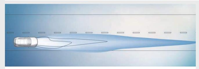
In laser high-beam mode, **BMW Laserlight with X Signature** illuminates a range of up to 600 m, nearly twice as far as that of conventional headlights. Better visibility in the dark significantly increases safety. The blue X signature and the "BMW Laser" lettering underline the vehicle's technological standards.
