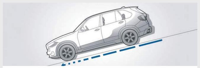
The **Hill Descent Control (HDC)** in the BMW X5 is a system which, when activated ensures that the vehicle can master the steepest downhill runs automatically and safely at just above walking pace, without the driver having to brake.
