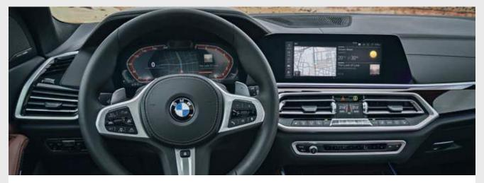
The **BMW Live Cockpit Professional** with navigation function includes a high-quality display network consisting of a high-resolution 31.2 cm (12.3 inches) Info Display that can be operated by touch and a fully digital 31.2 cm (12.3 inches) instrument cluster.
