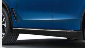
The **Aluminium running board** with a brushed, anodised surface and rubber inserts adds a particularly distinctive touch and makes getting in and out of the vehicle more convenient.
