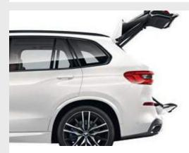
Both the upper and the lower part of the **Tailgate** can be opened and closed electrically. This facilitates access and loading of the luggage compartment.
