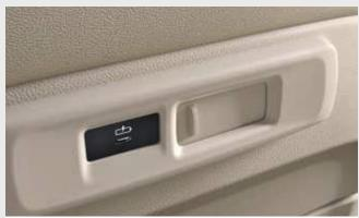
The **Travel & Comfort System** includes two additional USB ports (type C) and a preparation for two multifunctional holders in the rear of the vehicle. Tablets, clothes hangers or folding tables, for example, can be attached to them.
