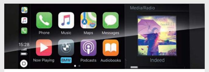
Preparation for **Apple CarPlay**<sup>®1,2</sup> supports the convenient and wireless use of selected iPhone® functions in the vehicle. This allows smartphone content and functions such as music, iMessages/text messages, telephony, Siri and selected third-party apps to be displayed and operated via the vehicle's user interface and via voice control.
