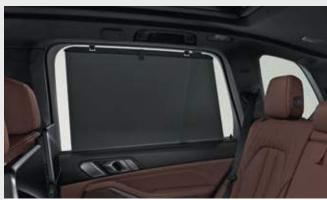
The manually operated **Roller Sunblind** for the rear side window protects the interior from sunlight and offers privacy.
