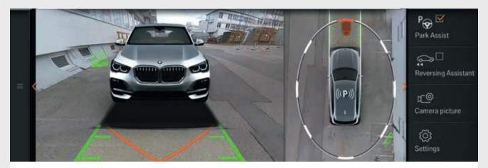
The Parking Assistant with Surround View Camera can handle the most difficult parking spots with ease. You can go in and out of parking spots with precision due to the system control the steering while you still have control of the accelerator, gears, and brakes. The Reversing Assistant supports you when reversing out of narrow lanes. Surround View includes rear view camera with Panorama View, Top View and 3D View.
