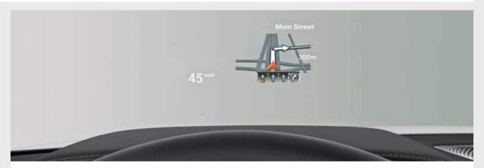
The full-colour BMW Head-Up Display projects all information relevant to the journey directly into the driver's field of vision, thereby allowing him to fully concentrate on driving. Information such as the current speed, navigation directions, along with telephone and entertainment information is displayed.
