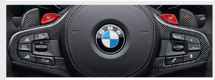
**M Performance Paddles, Carbon Fibre.** The M Performance paddles are covered with a very fine carbon fabric, finished in PUR paint and polished to a high gloss. The shift icons in M Red set additional motorsport highlights. Tiny details –fascinating impact.
