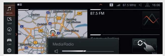
With BMW Gesture Control, certain functions can be operated by means of defined hand movements. For certain operations the system will for example recognise gestures such as swiping or pointing for accepting or rejecting an incoming call or circular motions of the index finger to adjust volume.
