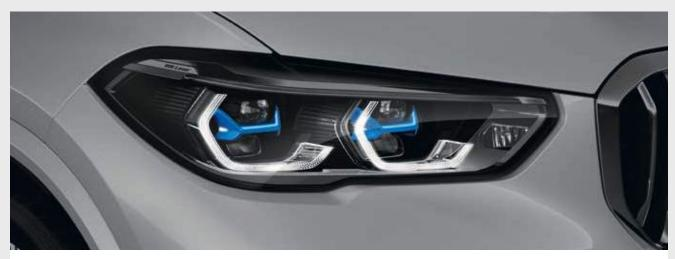
In laser high-beam mode, **BMW Laserlight with X Signature** illuminates a range of up to 600 m, nearly twice as far as that of conventional headlights. Better visibility in the dark significantly increases safety. The blue X signature and the "BMW Laser" lettering underline the vehicle's technological standards.
