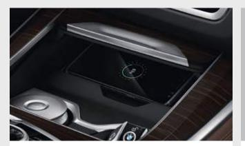
**Telephony with Wireless Charging** incorporates a wireless charging dock and a second microphone for a better hands-free voice quality. A roof aerial connection improves mobile reception. Two mobile telephones and an audio player can be connected simultaneously via Bluetooth.
